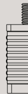
R6 (ADS7615) Fit 1-1/2 Square Tube Exp. 1.426 - 1.589 1/4 Square Metal Top Round Rubber 1/4 Square Metal Base
