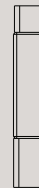
T2 (ATR7278) Fit 7/8 Square Tube Exp. 0.852 - 0.927 13/32 Square Top Square Rubber 3/4 Square Base
