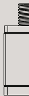
U5 (ADR7538) Fit 1-3/8 Square Tube Exp. 1.360 - 1.425 1/4 Square Metal Top Square Rubber 1/4 Metal Base
